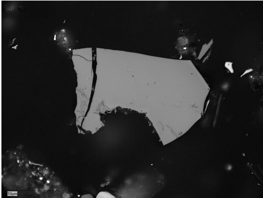
Figure 1: Coal grain; 50x objective, oil immersion, reflected white light.
