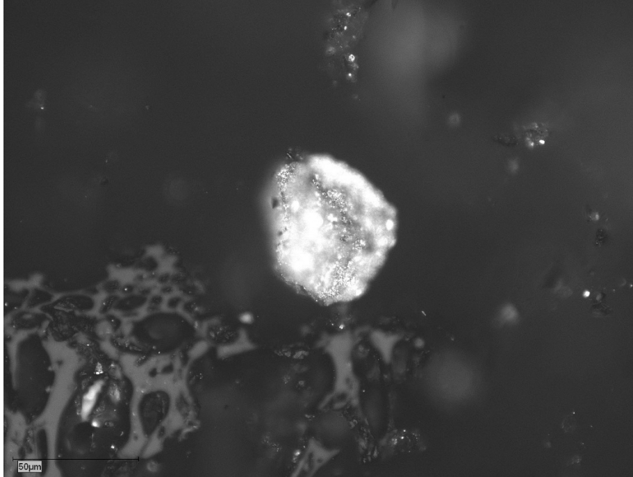
Figure 3: Mineral matter; 50x objective, oil immersion, reflected white light
