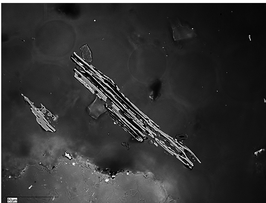
Figure 2: Organic material; 50x objective, oil immersion, reflected white light.
