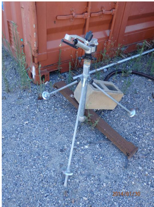
Figure 19: Relocatable sprinkler system
