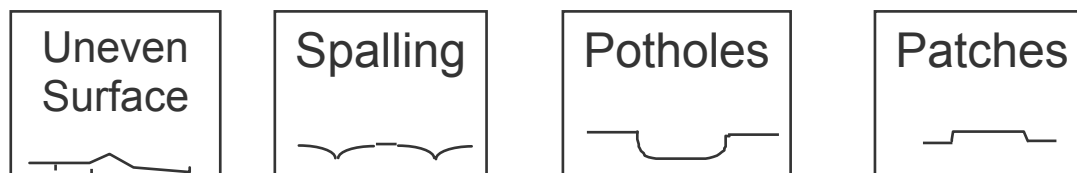
Figure 4 Road Surface Deformation Types and Cross Sectional Profile
