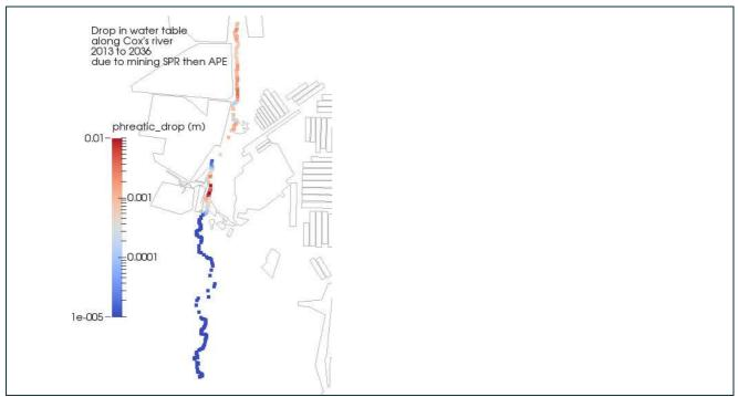
Figure G22 Drop in the phreatic surface along Cox's river between 2013 and 2036 due to mining APE and the new SV panels (SPR then APE scenario). A logarithmic scale has been used
