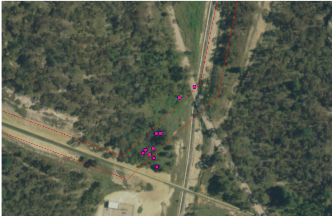
Figure 3 : Location of Eucalyptus aggregata trees (pink dots) in the project application area in the location where the pipeline was realigned to allow for HDD in order to eliminate the right angle bend
