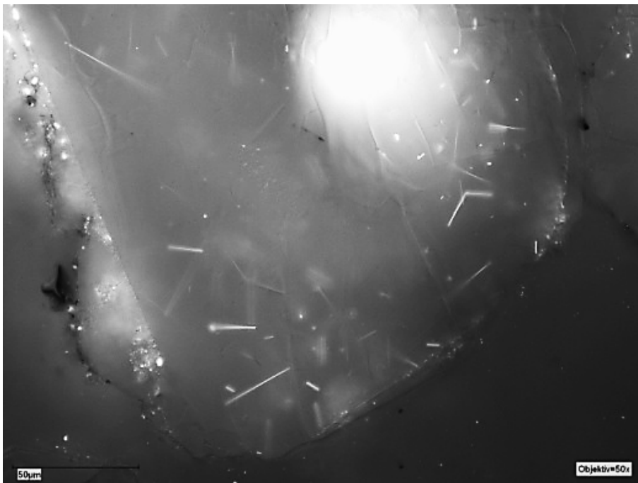
Figure 4: Mineral matter; 50x objective, oil immersion, reflected white light
