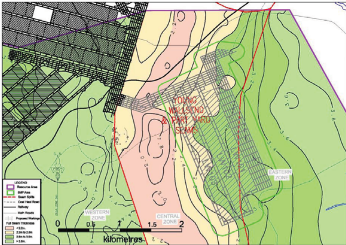
Fig. 1.11 Target Seam Thickness Contours (Newstan, 2011)
