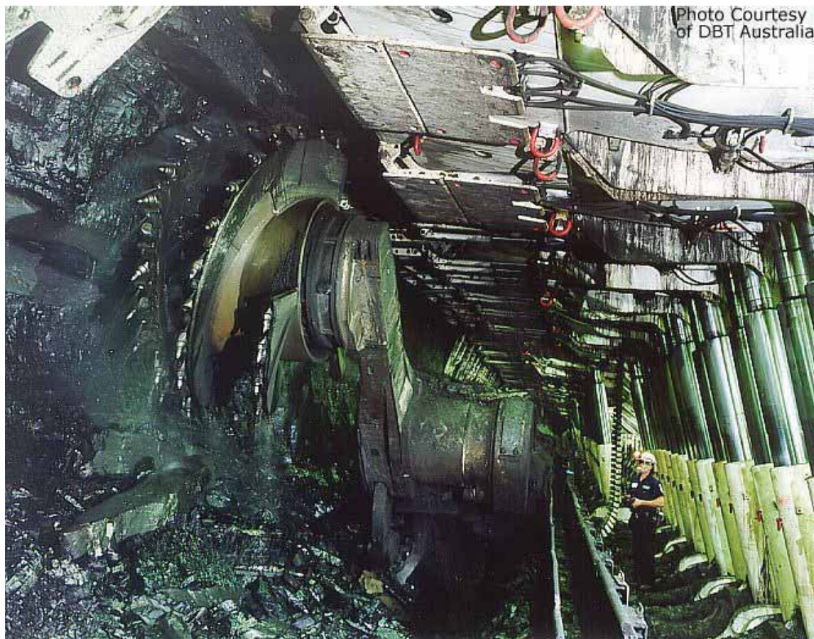
Fig. 3.2 An Operating Longwall Face
